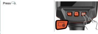
The function assigned to the quick select button is carried out.
