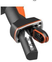
3 Close the battery compartment cover and secure with the unlocking button.
